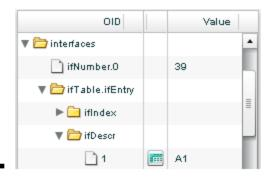
10. To view the MIB table of multiple instances, click the <sup>IIII</sup> View MIB Table button or select a row that contains a <sup>IIII</sup> View MIB Table button and click **View** → **MIB Table**.
