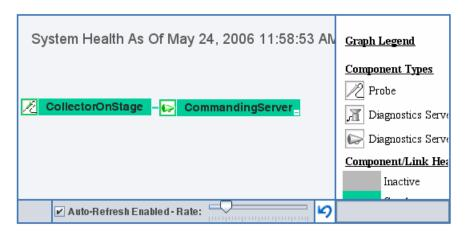
When the Collector is stopped, the Collector node in the System Health monitor is gray. When the Collector starts, the node is green.
