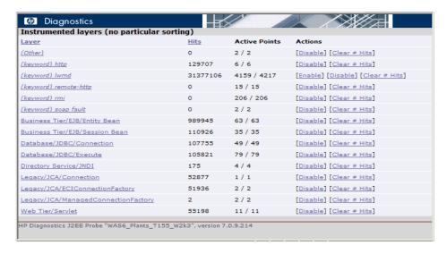
To disable a layer from the Instrumented Layers page, click the **Disable** link associated with the layer on the page. The layer is disabled and the link toggles to **Enabled** so that you can enable the layer again when necessary.
