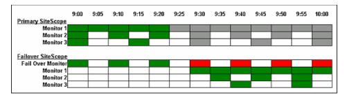
In the figure above, the upper table represents three monitors running on a primary SiteScope. Monitor 1 runs every five minutes, Monitor 2 runs every ten minutes and Monitor 3 runs every 15 minutes. At some time between 9:20 and 9:25, the primary SiteScope became unavailable. The grey squares indicate what would have been the monitor runs executed if the primary had not failed. These are included to illustrate the measurement data gap and offset.
