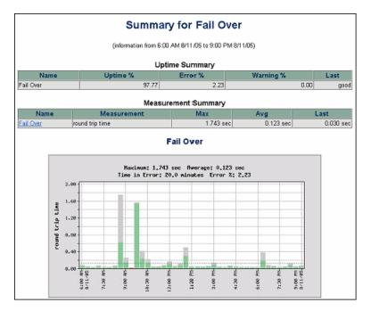
The other tables on the chart give a more explicit indication of the failover activation event. The following figure is an example of the listing of error readings made by the Fail Over monitor. This table is normally displayed in the lower portion of the report page.
