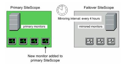
As installed, SiteScope Failover is set to query the primary SiteScope every four hours. The following figure illustrates the automated mirroring operation which copies the configurations to include the newly added monitor to the failover machine. You can configure the frequency of the mirroring on the failover installation.
