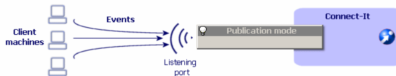
Figure 9-10: XML listening connector in publishing mode
