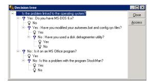
Select a node in the tree and click the **Access** button to change the starting node of the branch on which you want to work. You will need to use this technique to avoid having to navigate through the entire branch at a given moment.
