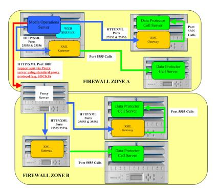
Figure 23 Media Operations deployment options with Data Protector
