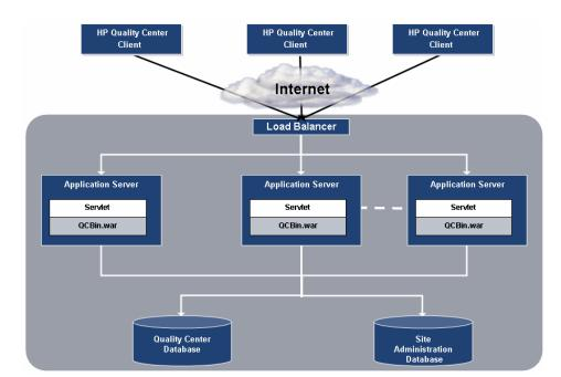
The following diagram illustrates how Quality Center client requests are transmitted within a cluster.
