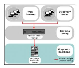
**Note:** Different types of reverse proxies require different configuration syntaxes. For an example of an Apache 2.0.x reverse proxy configuration, see "Apache 2.0.x – Example Configuration" on page 305.
