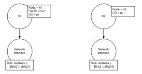
In this example, the input node matches two nodes in the CMDB having different identification criteria, and there are conflicts with the CMDB matched nodes.
