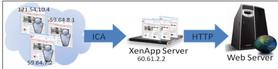
When monitoring the Web server with Real User Monitor, it is desirable to see the real end users as the clients, rather than having a single client combining all the traffic. To achieve such functionality, you must install the RUM HTTP Agent on the XenApp server.
