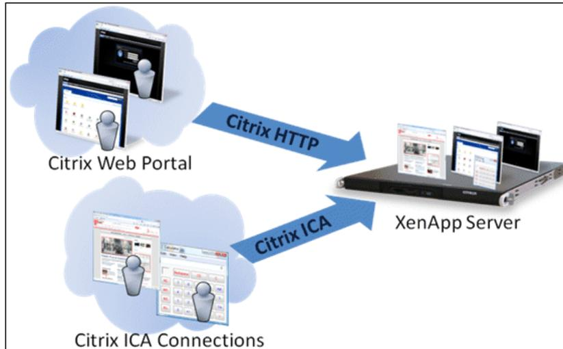
An end user starts by opening a Citrix Web portal and selecting one of the published applications. An ICA session is created, in which the selected application runs on the XenApp server, and the user uses the application remotely.
