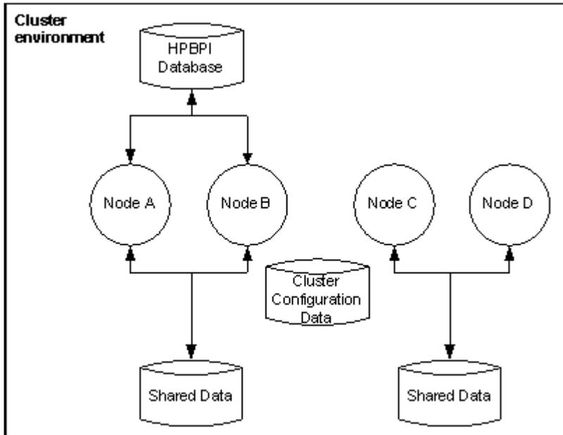
In order for the failover to be successful, both Node A and Node B must have access to the BPI data. This includes the installation data and configuration files on disk, plus all the Process, Monitor and Events data in the database. In this diagram it is only Nodes A and B that have this access. Nodes C and D are also operating in the cluster but are not available for BPI failover.
