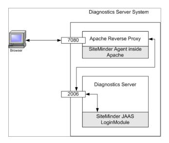
In the above diagram, an Apache web server listening for requests on port 7080 is configured as a reverse proxy. It contains the SiteMinder web agent which performs the authentication and if successful, allows Apache to pass the request through to port 2006 (or whatever Diagnostics Server port is configured) on which the Diagnostics server listens.
