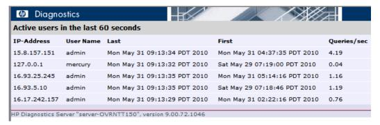
You can configure limits on the queries the UI is executing if you find there are very high query loads. Use the **ui.properties** file on the server to set properties to throttle update frequency of ui queries to the server.
