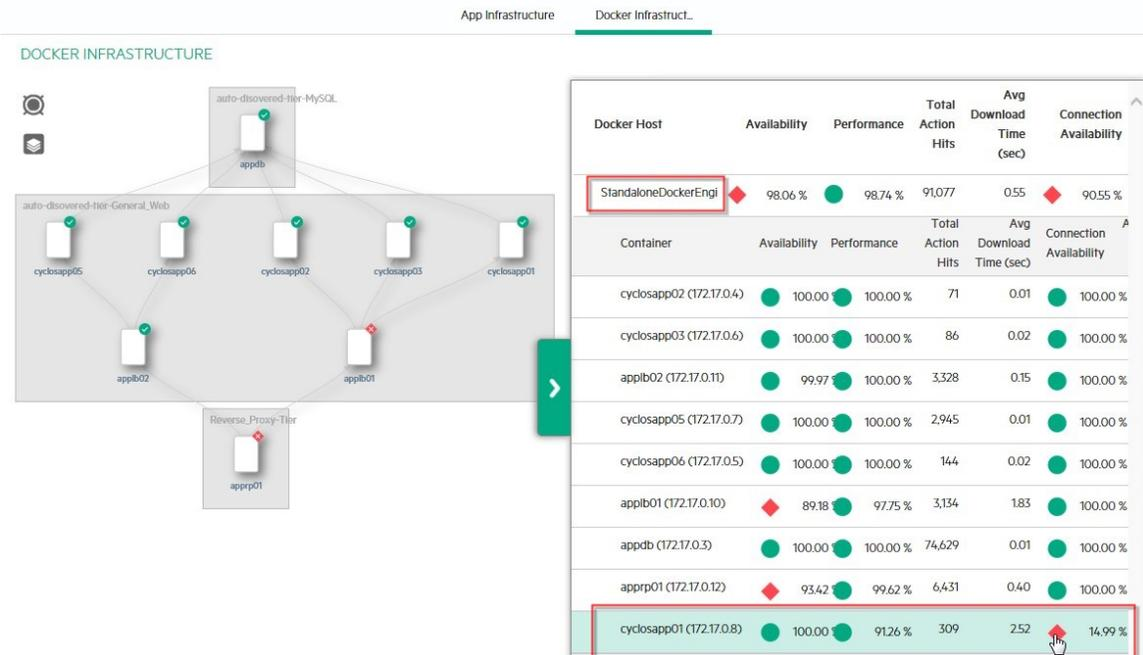
The only remaining action is to resolve the problem by recreating or fixing the affected root-cause container **cyclosapp01** that is hosted on the Docker Engine **StandaloneDockerEngine**.
