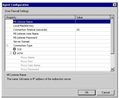
5. For the **Local Machine Key** property, enter the machine name of the host of the Diagnostics mediator server.
