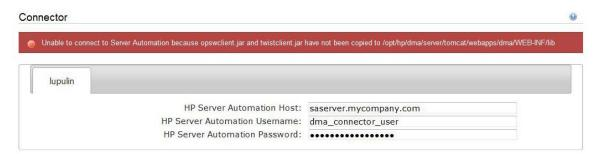
If you receive this error message, verify the contents of the /var/log/hp/dma/dma.log file. If the file contents are similar to the following, the opswclient.jar and twistclient.jar files are not at the required locations:
