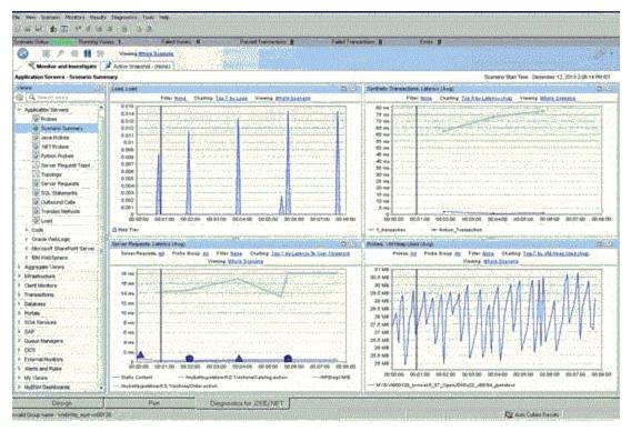
Once you are in the Diagnostics UI you can navigate to other views to identify, isolate, analyze, and solve performance problems detected during the run.
