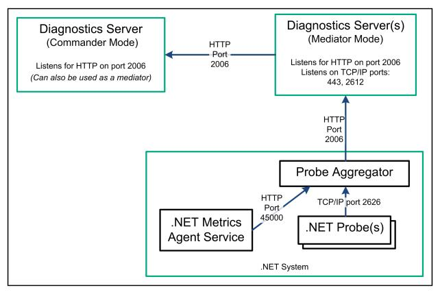
The Probe Aggregator Service aggregates probe data to 5 second intervals before sending the performance data to the Diagnostics mediator server. This is useful when the volume of data collected based on instrumentation of multiple applications is high and networking traffic would be too great if not aggregated.
