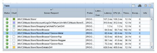
The **httppcaptureparams** element can also be used to capture the original URI of the server request. To capture the unmodified server request, set the **capturequerystring** argument to true:
