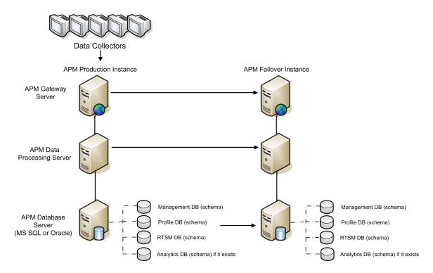
In the example above (with no external UCMDB) database replication is used to replicate all of the APM databases. In the next example, there is an external UCMDB as the topology system of record. Therefore, only the Management and Profile databases are replicated. Topology synchronization from the external UCMDB keeps the RTSM databases synchronized.
