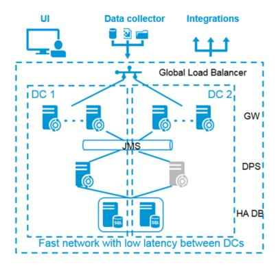
A more detailed implementation diagram is shown below. This shows the APM Gateway servers and APM Data Processing Servers split across the two different data centers. A database cluster is also housed with nodes in each data center. The APM Database acts as a single database clustered across two different physical locations.
