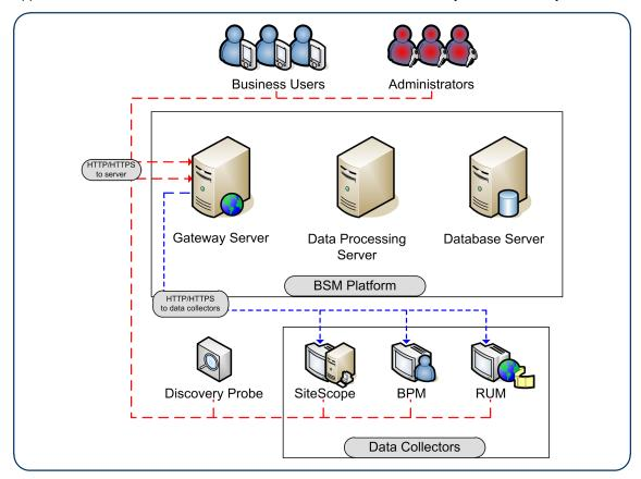
Application users / data collectors that communicate with APM Gateway Servers using Reverse Proxy.
