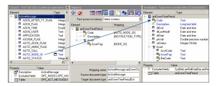
The link can be made by dragging the source element and dropping it on the destination element.
