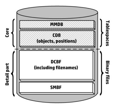
The MMDB and CDB parts are implemented using an embedded database consisting of tablespaces. This database is controlled by the hpdp-idb, hpdp-idb-cp, and hpdp-as processes. CDB (objects and positions) and MMDB present the core part of IDB.
