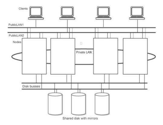
As shown in the figure, an HACMP cluster is made up of the following physical components:
