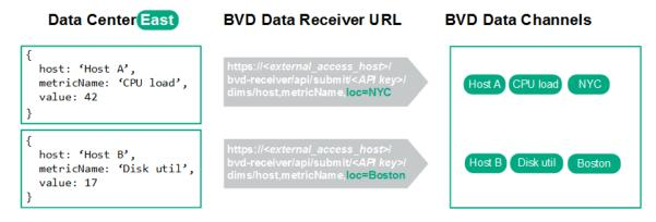
The primary location of Data Center East is in New York City, with backup servers located in Boston. Both locations send the same set of JSON data. To differentiate the data from the two locations without modifying the JSON data, you can add an additional dimension loc with the corresponding value to the URL. The modified URL updates the data channels to
