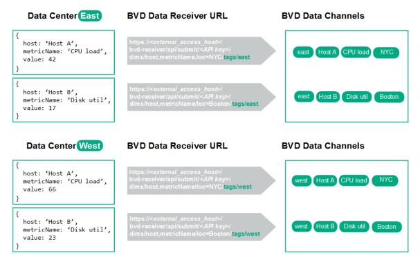
A second data center, Data Center West, starts sending data similar to the JSON data sent by Data Center East. The data from Data Center West uses the same data channels as the data from East. To distinguish the data from the two centers, you must add the origin to the data. You can do this by adding tags to the URL. Tags are static labels that you can attach to your data to create more specific data channels.
