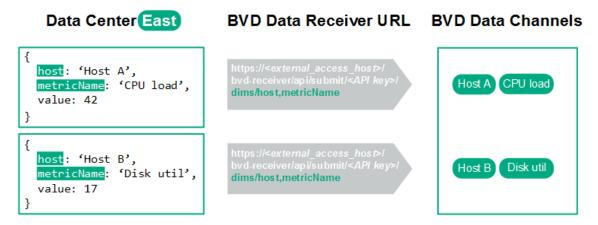
In this example, Data Center East sends two sets of JSON data to the BVD receiver. In both sets, the data fields host and metricName uniquely identify the value. The fields are therefore selected as dimensions (dims) and included in the URL. Once received by the BVD server, the JSON data creates two data channels:
