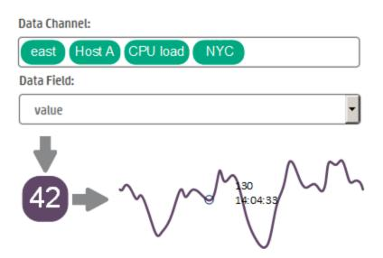
Once BVD has received the data, it creates the corresponding data channels. You can then associate a data channel with your widget in the widget's properties. In this example, the data channel east the Host Att CPU load NYC has been selected for the sparkline widget.
