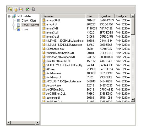
This example displays the contents of the Microsoft Applications Center 2000 SP2 installer. The same installer contains both Server and Client components of the application.
