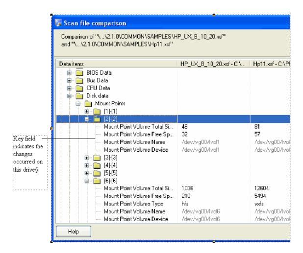
The Mount Point Volume Name field is a key field (shown in grey) and this is shown even though it hasn't changed itself. This indicates that the information changed relates to this particular drive; without the key field it would not be possible to see on which drive the change had taken place, merely that it had changed on some drive.
