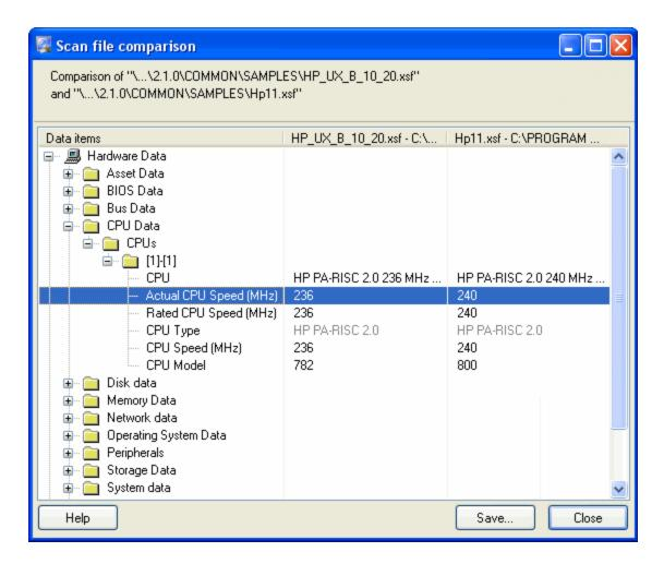
In this example, the Actual CPU Speed for the first scan file is 236 MHz and 240 MHz for the second scan file.
