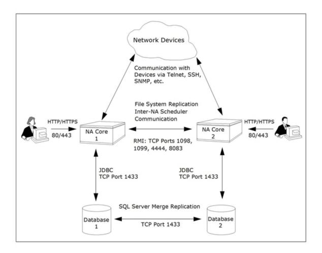
Keep in mind that some installations might have two separate network device collections that are inaccessible from the non-managing NA Core. These installations still provide data redundancy and scaling benefits, however.
