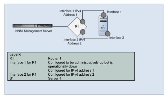
**Scenario**: Interface 1 is operationally down (if0perStatus = down) and administratively up (ifAdminStatus = up). Router 1 sends a linkDown trap. Router 1 can be reached because some IP addresses, such as IP Address 2, respond to ping. The SNMP agent is up. IP Address 1 is associated with Interface 1. IP Address 1 has stopped responding to ICMP.
