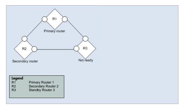
**Scenario**: The Router Redundancy Group has had some change. The group is functioning, and there are one primary router and one secondary router, but there is some non-normal condition that could be an issue. For example, there might be several routers not in a Standby state.
