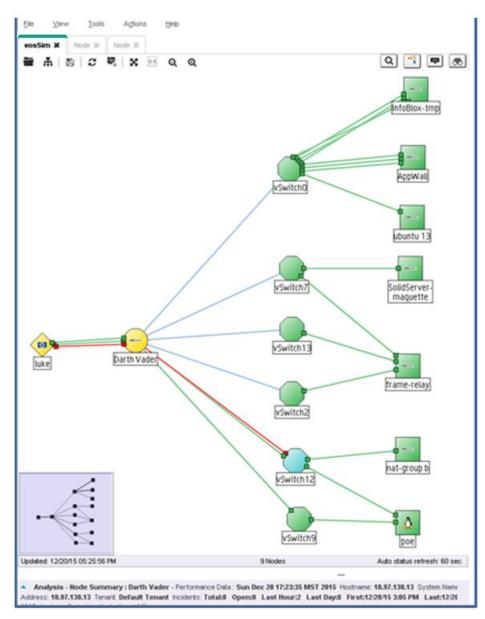
**Scenario**: (*NNMi Advanced*) A connection between the hypervisor and access switch is down.
