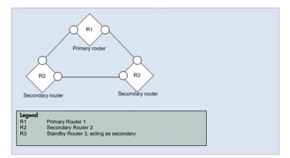
**Scenario**: A Router Redundancy Group has multiple routers reporting as the secondary router. A properly functioning HSRP or VRRP Router Redundancy Group should have only one operational secondary router.
