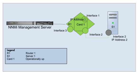
**Scenario**: This scenario continues the previous "Card is Operationally Down" scenario. Card 1 is operationally up (card0perStatus = up). The node (Router 1) can be reached and all of its IP addresses respond to ping. The card is up and all the interfaces and connection on Card 1 are back to normal. The SNMP agent is up.
