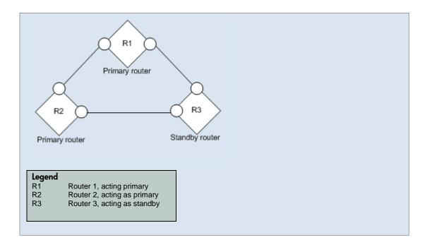
**Scenario**: A Router Redundancy Group has multiple routers reporting as the primary router. A properly functioning HSRP or VRRP Router Redundancy Group should have only one operational primary router.
