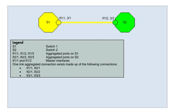
Scenario: Some (but not all) ports within the port aggregator are operationally down.
