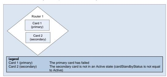
**Scenario**: A Card Redundancy Group does not have a primary member. The cardStandbyStatus of the primary card (Card 1) is not Active. Router 1 sends a CiscoRFProgressionNotif or a CiscoRFSwactNotif trap on the Card Redundancy Group state changes.
