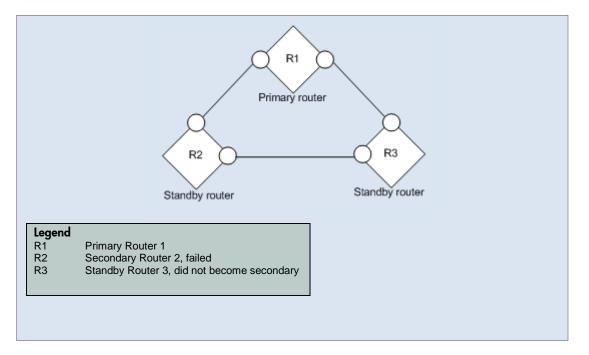
**Scenario**: A Router Redundancy Group has had a failure on the secondary router. Either there is no standby, or the standby did not take over as the secondary.
