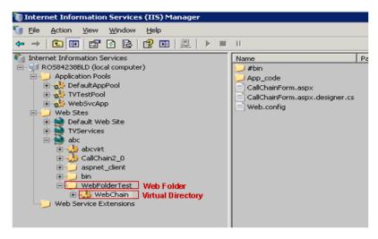
Because of an issue with the WMI provider, the listing in WMI for this web site would not show the WebFolderTest/WebChain virtual directory. The .NET Agent uses the listing from the WMI provider to discover web applications. So in situations like this, the .NET Agent may not be able to discover virtual directories under a web folder.
