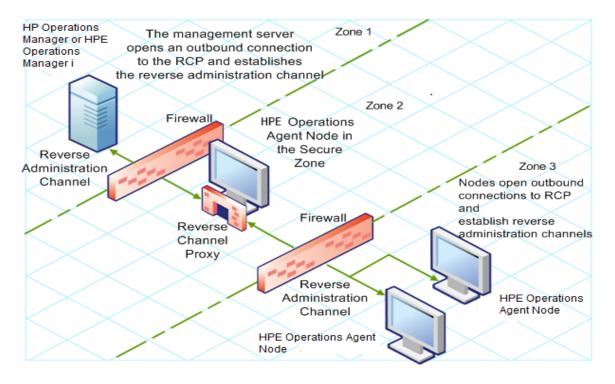
In this scenario, you must install the agent on a system in the intermediate zone (zone 2) and configure the RCP on the system. After you configure the nodes in the zone 3 and the management server in the zone 1 to establish reverse administration channels to the RCP, server-node bidirectional communication takes place through the RCP.
