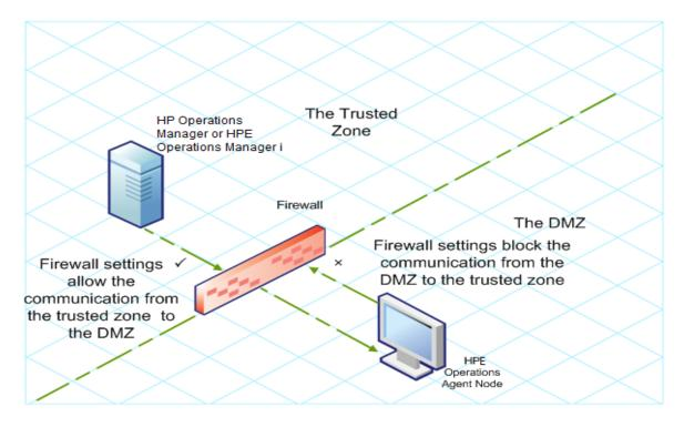
In the following scenario, managed nodes are located in the trusted zone while the management server belongs to the DMZ. The firewall settings in this example allow outbound-only communication from the node to the HPOM or the HPE OMi management server, but block the inbound communication to node.
