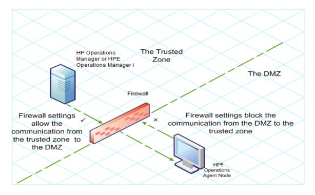
When the nodes are located in the trusted zone and the management server in the DMZ, the HPOM or the HPE OMi setup uses the following workflow:
