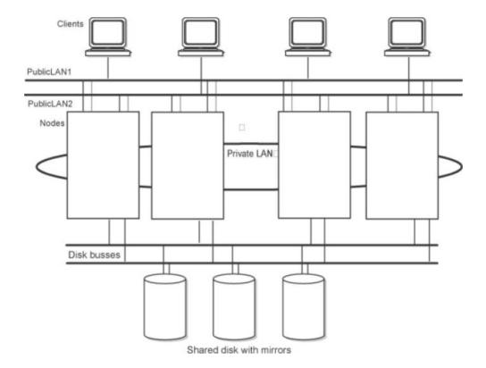
As shown in the figure, an HACMP cluster is made up of the following physical components:
