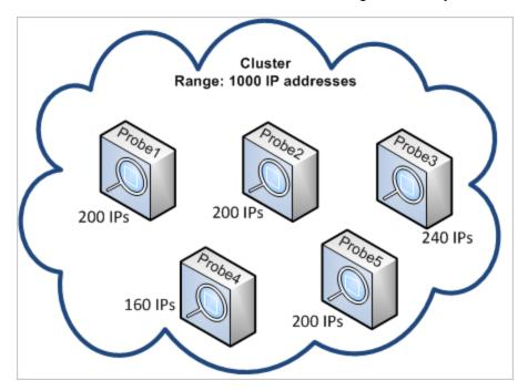
If, however, there are Probes with less than 160 IPs, or more than 240 IPs (see image below)—that is, more than a 20% deviation from the average 200—the cluster attempts to re-balance the IPs among the Probes—as long as the TQL constraints on the Probes allow this.
