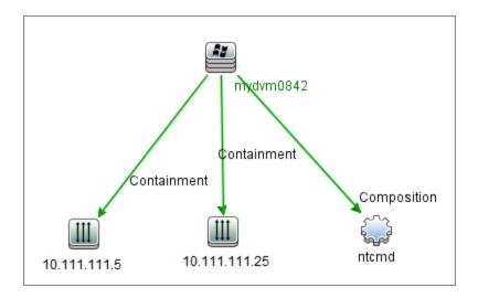
Only one of these IP addresses is recorded in the Protocol CI in the Application IP attribute, which **mydvm0842** then uses for communicating with the Data Flow Probe and for determining which Management Zone **mydvm0842** will belong to.
