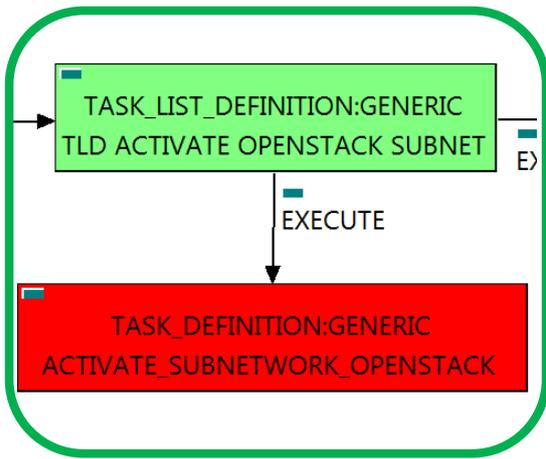
The TDs that have present in the their names “Activate”, are Task Definitions responsible of the activation in the platform targeted and the updating of the status in the platform and the DDBB, in this case, the artifact that is going to be activated is a “SUBNETWORK:OPENSTACK”, this means, when this workflow finish, we will have a SUBNETWORK:OPENSTACK with status ACTIVE identified as part of the Service Network.
