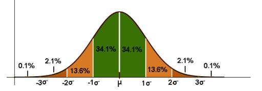
The script compares the current data average with the standard deviation levels, to determine if the current data exceeds or precedes either one standard deviation or two standard deviations of the baseline data.
