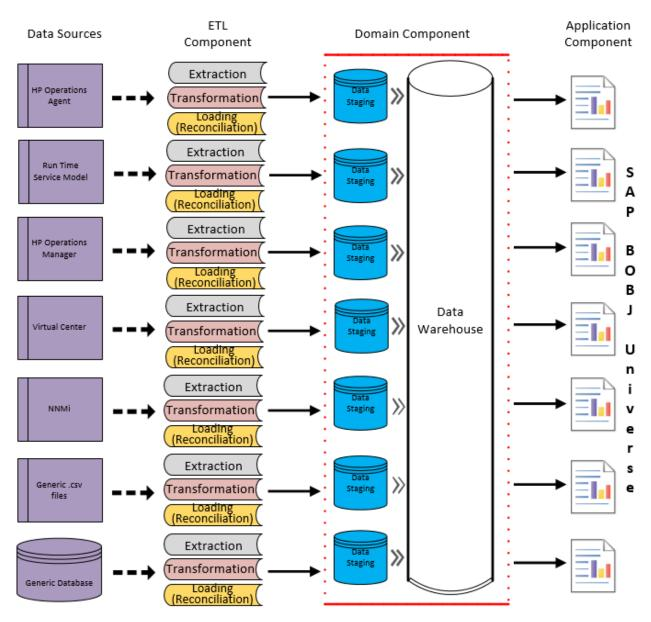
The following figure shows the typical data flow between the components of the Content Pack:
