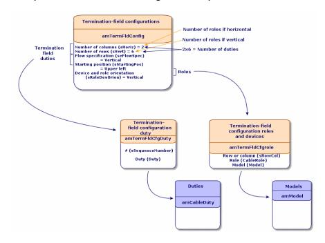
Example of termination-field configuration - correspondence at the termination field level
