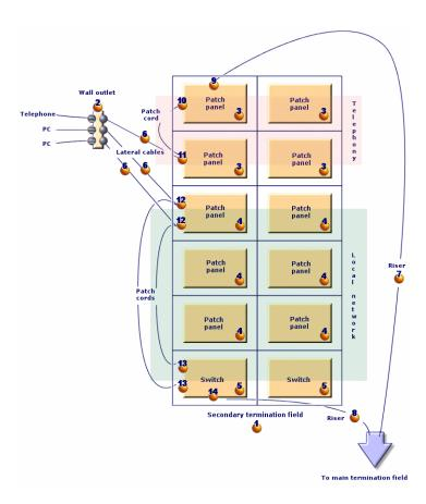
This network contains components that will not be used in the example illustrating the Cable and Circuit module:
