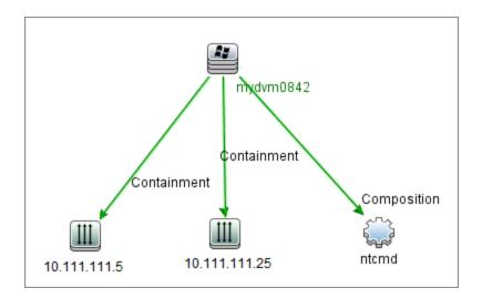
Only one of these IP addresses is recorded in the Protocol CI in the Application IP attribute, which **mydvm0842** then uses for communicating with the Data Flow Probe and for determining which Management Zone **mydvm0842** will belong to.
