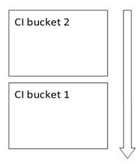
The multithreaded Data-In service concurrently processes multiple CI buckets on multiprocessor or multi-core systems if these buckets do not carry overlapping CIs.
