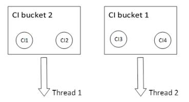
To guarantee the data model consistency, the multithreaded Data-In service processes the CI buckets that carry the same CI information sequentially. In this situation, the multithreaded architecture does not improve the performance of the Data-In service.
