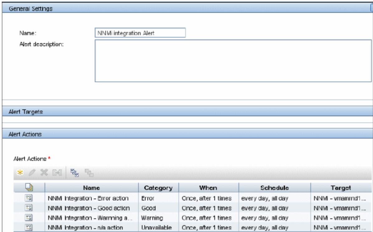
3. When an alert is triggered in SiteScope as a result of a monitor status change, the alert reports an SNMP trap to the NNMi management server. NNMi reads the SNMP trap, translates the attributes, and displays the SiteScope event data in NNMi's **Incident Browsing** workspace.
