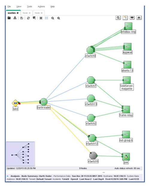
**Scenario**: (*NNMi Advanced*) All Up Link interfaces on a virtual switch have been administratively downed by a network operator.
