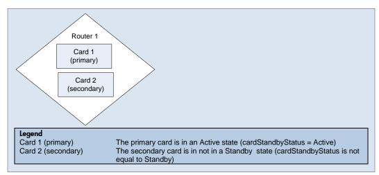
**Scenario**: A Card Redundancy Group does not have a secondary member. Neither card has a cardStandbyStatus equal to Standby. A properly functioning Card Redundancy Group should have one operational primary card and one operational secondary card.
