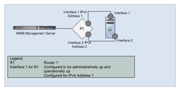
**Scenario**: This scenario continues the previous "Interface is Administratively Down" scenario. Interface 1 on Router 1 is now administratively up (ifAdminStatus = up). Some of the IP addresses of that interface respond to ping. The SNMP agent is up. Enabling Interface 1 on Router 1 brings it operationally up. The IP address associated with this interface starts responding to ICMP.
