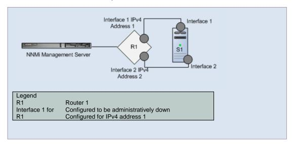
**Scenario**: Interface 1 on Router 1 is administratively down (ifAdminStatus = down), but the node (Router 1) can be reached. For example, Interface 2 responds to ping and the SNMP agent is up. Disabling Interface 1 brings that interface operationally down. The IP address associated with this interface, IP Address 1, stops responding to ICMP.
