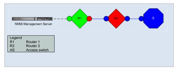
Scenario: There is no redundancy to Router 2 (R2). Either Router 2 is down or the connection between Router 1 (R1) and Router 2 is down.
