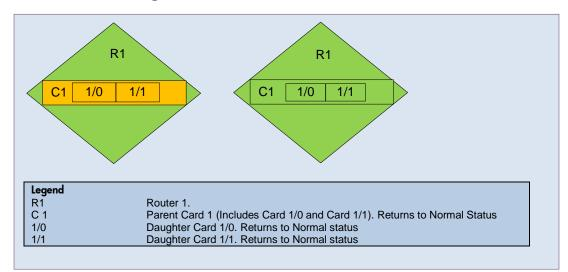
**Scenario**: This scenario continues the previous "Parent Card Management Mode is Unmanaged or Out-of-Service" scenario. The Parent Card management mode is now set to Inherited. This means the Parent Card's management mode is inherited from its container node (Router1), which is Managed.
