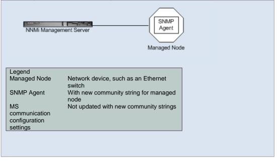
**Scenario**: The SNMP agent is not responding. For example, the community string for this SNMP agent has been changed, or NNMi's communication configuration settings have not yet been updated, but the node is operational (IP addresses can be pinged).
