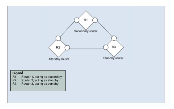
**Scenario**: A Router Redundancy Group does not have a primary member. A properly functioning HSRP or VRRP Router Redundancy Group should have one operational primary router and one operational secondary router.
