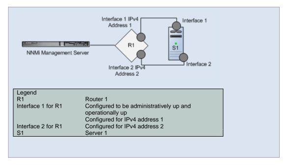
**Scenario**: This scenario continues the previous "Interface is Operationally Down" scenario. Interface 1 on Router 1 is now operationally up (if0perStatus = up). The node can be reached. All of its IP addresses respond to ping. The SNMP agent is up.
