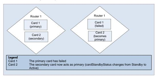
**Scenario**: A Card Redundancy Group has a failure on the primary card. The cardStandbyStatus on the secondary card changes from the value of Standby to Active. This Active card takes over as the primary member. In this case, the Card Redundancy Group is functioning as intended.
