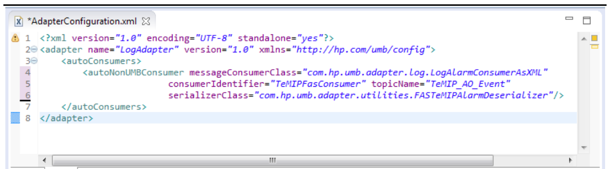
Figure 8 - Example of autoNonUmbConsumer flow definition in the AdapterConfiguration.xml file
