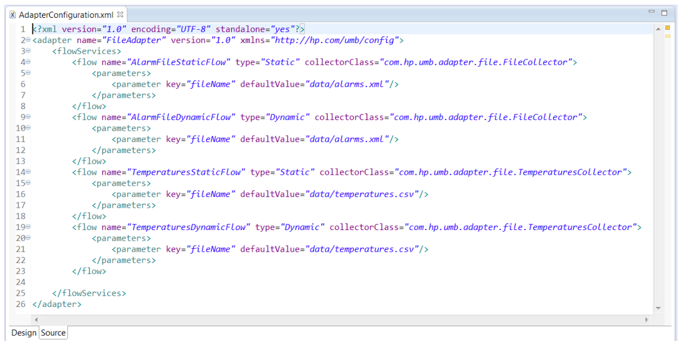
Figure 55 - The File Adapter's AdapterConfiguration.xml file
