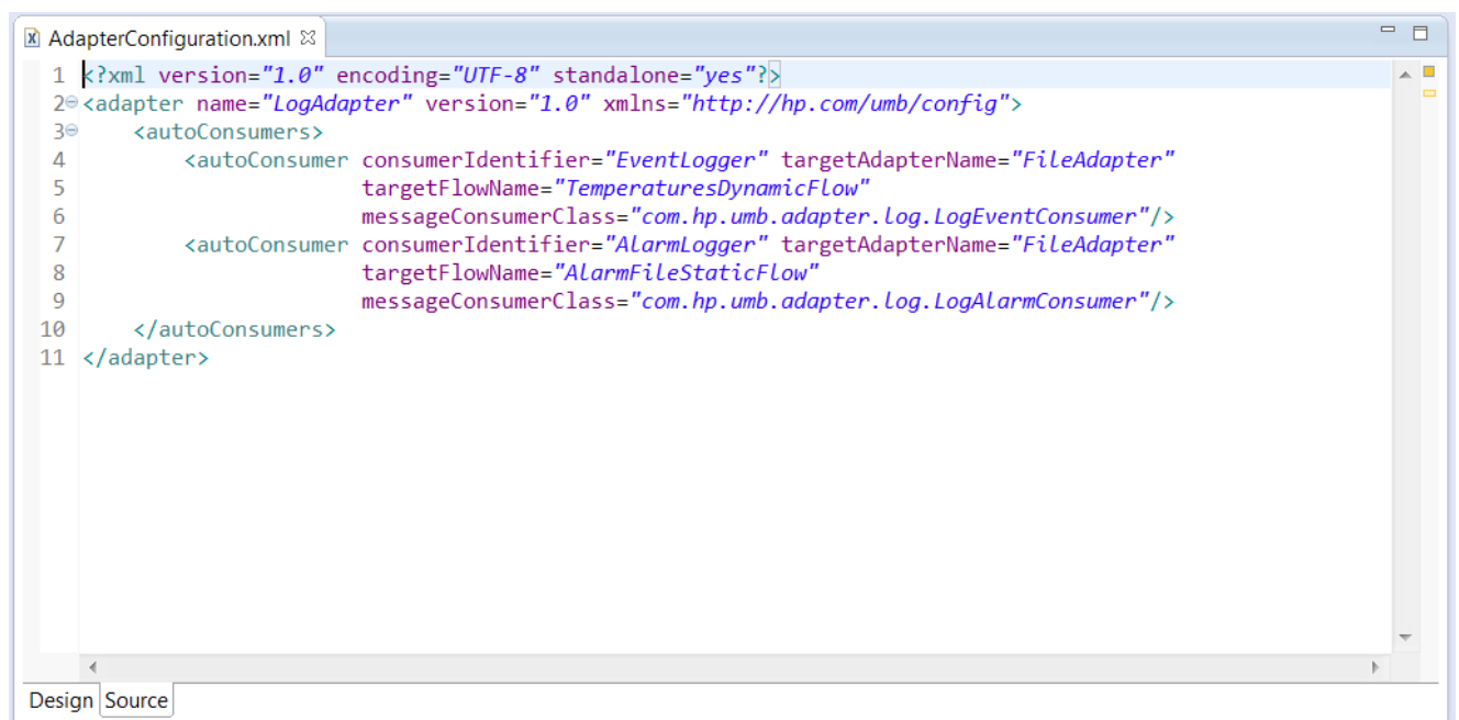
Figure 61 - The Log Adapter's AdapterConfiguration.xml file
