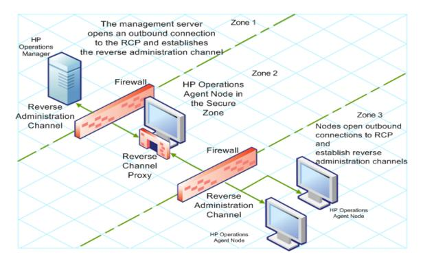
In this scenario, you must install the agent on a system in the intermediate zone (zone 2) and configure the RCP on the system. After you configure the nodes in the zone 3 and the management server in the zone 1 to establish reverse administration channels to the RCP, server-node bidirectional communication takes place through the RCP.
