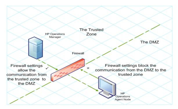
When the nodes are located in the trusted zone and the management server in the DMZ, the HPOM setup uses the following workflow:
