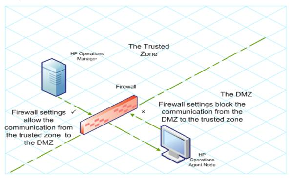
In the following scenario, managed nodes are located in the trusted zone while the management server belongs to the DMZ. The firewall settings in this example allow outbound-only communication from the node to the HPOM management server, but block the inbound communication to node.
