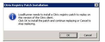
Due to limitations in Citrix, a Citrix script may not run successfully in server mode, but will run successfully in process mode. • You should also confirm that a separate user session is not running the Citrix Connection Center, outside of BPM. To resolve this issue, close all instances of concenter.exe and other citrix processes for all users.
