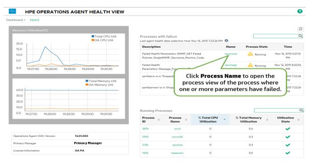
Check the Health Parameter details. The health parameter corresponding to the source (as per policy) from where the process is unable to collect data will show the status as failed. For example, the status of the health parameter SNMP GET is Failed.
