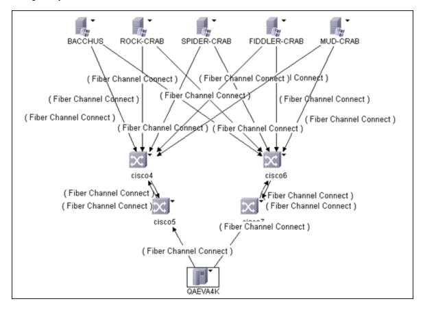
The following diagram illustrates the SAN Topology and shows the fiber channel paths between storage arrays, switches, and servers:
