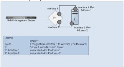
**Scenario**: IP address 1 on Server 1 (S1) is not responding. For example, the route on Router 1 (R1) has changed from Interface 1 to Interface 2, so that packets destined for the interface 1 on Server 1 are now routed out of Interface 2 on Router 1. The associated interface is operational, and the node can be reached because you can ping some IP addresses. The SNMP agent is up.
