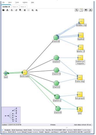
Scenario: (NNMi Advanced) Web Agent on hypervisor is not responding. For example, there is an issue with the hypervisor hosting the Web Agent, and the agent is no longer responding to requests for state information from NNMi but the hypervisor node is operational (IP addresses can be pinged).
