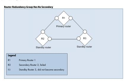
**Scenario**: A Router Redundancy Group has had a failure on the secondary router. Either there is no standby, or the standby did not take over as the secondary.
