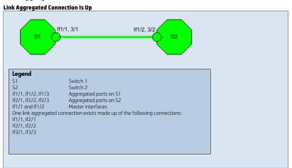
**Scenario**: All port aggregator members of the connection are up. **Root Cause**: The aggregator is up on all members of the connection.
