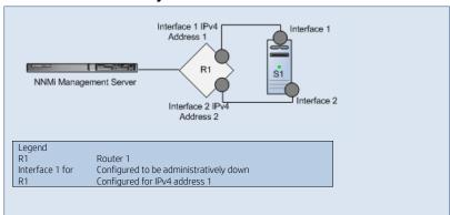
Scenario: Interface 1 on Router 1 is administratively down (ifAdminStatus = down), but the node (Router 1) can be reached. For example, Interface 2 responds to ping and the SNMP agent is up. Disabling Interface 1 brings that interface operationally down. The IP address associated with this interface, IP Address 1, stops responding to ICMP.
