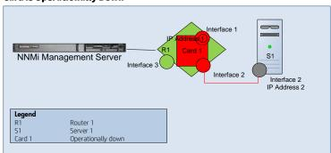
Incident: A CardDown incident is generated. The moduleDown or CiscoModuleStatusChange incident is correlated under the CardDown incident. The InterfaceDown incident for Interface 1 and the ConnectionDown incident between Interface 2 on Router 1 (R1) and Interface 2 on Server 1 (S1) are correlated under the CardDown incident. The InterfaceDown incident for Interface 2 is correlated under ConnectionDown.
