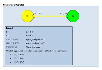
Scenario: Some (but not all) ports within the port aggregator are operationally down.
