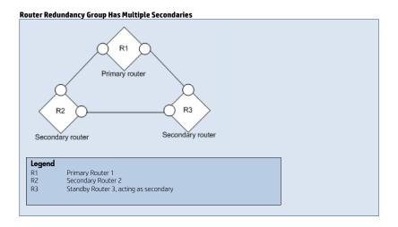
**Scenario**: A Router Redundancy Group has multiple routers reporting as the secondary router. A properly functioning HSRP or VRRP Router Redundancy Group should have only one operational secondary router.
