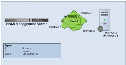
**Scenario**: This scenario continues the previous "Card is Operationally Down" scenario. Card 1 is operationally up (cardOperStatus = up). The node (Router 1) can be reached and all of its IP addresses respond to ping. The card is up and all the interfaces and connection on Card 1 are back to normal. The SNMP agent is up.
