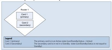
**Scenario**: A Card Redundancy Group does not have a secondary member. Neither card has a cardStandbyStatus equal to Standby. A properly functioning Card Redundancy Group should have one operational primary card and one operational secondary card.
