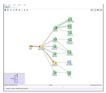
Scenario: (NNMi Advanced) Multiple connections between the hypervisor and access switch are down.
