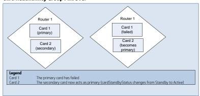
**Scenario**: A Card Redundancy Group has a failure on the primary card. The cardStandbyStatus on the secondary card changes from the value of Standby to Active. This Active card takes over as the primary member. In this case, the Card Redundancy Group is functioning as intended.
