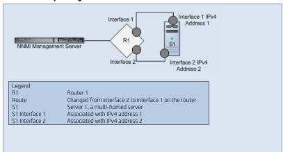
**Scenario**: This scenario continues the previous "IP Address Not Responding to ICMP" scenario. The IP address is now responding, the associated interface is operational, and the node can be reached. (For example, you can ping some IP addresses and the SNMP agent is up, or both.)
