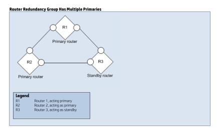
**Scenario**: A Router Redundancy Group has multiple routers reporting as the primary router. A properly functioning HSRP or VRRP Router Redundancy Group should have only one operational primary router.
