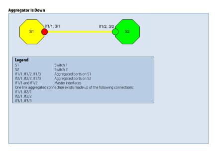
$\textbf{Scenario} \hbox{: All ports within the port aggregator are operationally down.}$
