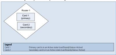
**Scenario**: A Card Redundancy Group has both members reporting as the primary card. The cardStandbyStatus of both cards is Active. A properly functioning Card Redundancy Group should have only one operational primary card.
