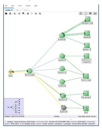
Scenario: (NNMi Advanced) All Up Link interfaces on a virtual switch have been administratively downed by a network
