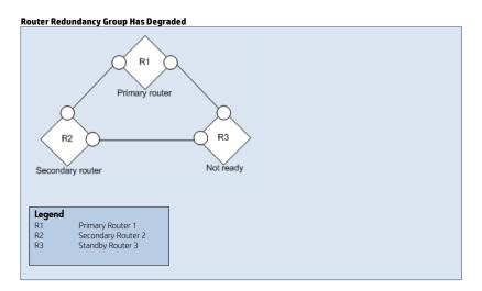
**Scenario**: The Router Redundancy Group has had some change. The group is functioning, and there are one primary router and one secondary router, but there is some non-normal condition that could be an issue. For example, there might be several routers not in a Standby state.
