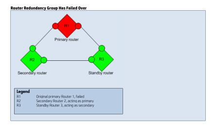
**Scenario**: A Router Redundancy Group has had a failure on the primary router and the secondary router has taken over as primary. Usually the standby becomes the secondary, which is not a problem. The group is functioning as intended. The incident generated for this scenario is for informational purposes to report that the group has had a failover.
