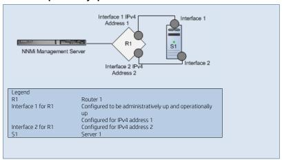
**Scenario**: This scenario continues the previous "Interface is Operationally Down" scenario. Interface 1 on Router 1 is now operationally up (ifOperStatus = up). The node can be reached. All of its IP addresses respond to ping. The SNMP agent is up.
