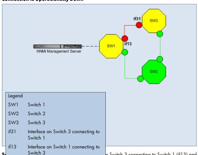
Switch 3 n Switch 3 connecting to Switch 1 (if13) and the interface on Switch 1 connecting to Switch 3 (if31) is down. Traffic flows from the Management Server through Switch 1 (SW1) and Switch 2 (SW2). Both if13 and if31 are marked down.
