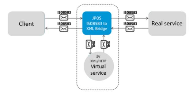
Service Virtualization provides an external extension based on jPOS that works with an XML virtual service. The Service Virtualization ISO 8583 jPOS bridge converts ISO 8583 messages into XML and passes them back and forth between jPOS and Service Virtualization.
