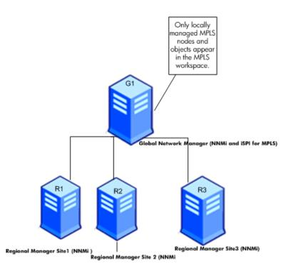
In this deployment scenario, only the locally managed MPLS nodes and objects such as L3 VPNs, L2VPNs, MVPNs, and PseudoWire VCs are available in the MPLS inventory (G1).
