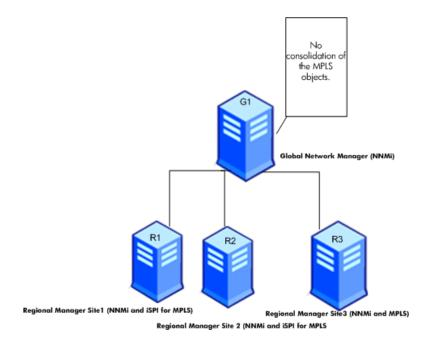
In this deployment scenario, all the Regional Managers (R1, R2, and R3) discover the MPLS nodes and objects such as VRFs, TE Tunnels, VC LSPs, and MVRFs. The NNM iSPI for MPLS is not available on G1 so there is no communication established between G1 and regional managers for the NNM iSPI for MPLS. Thus, the MPLS nodes and objects from the Regional Managers are not available in the G1 inventory. In addition, no aggregated MPLS reports are available in the MPLS (GNM) inventory.
