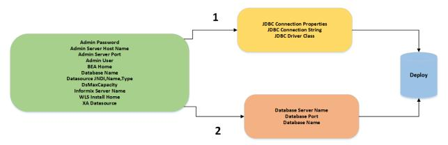
Path 2: This is used to create a datasource with the JDBC drivers which are part of the standard WebLogic installation. The JDBC connection string is constructed from the user given values to the three parameters as shown. Path 1: This is used to create a datasource with the third party JDBC drivers which are installed by the user in their WebLogic environment.
