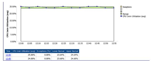
3. When the NNM iSPI Performance for Metrics detects a metric value that lies outside of the baseline sleeve for 15 minutes or longer within the last 30-minute window, the NNM iSPI Performance for Metrics raises an exception and sends an incident to the NNMi Incident View. You can view these exceptions on a Chart Detail report by selecting the CPU 1Min Utilization - Baseline Exception Count metric.
