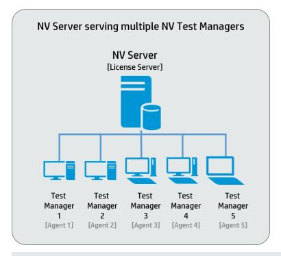
Note: The NV Server and the NV Test Manager cannot be installed on the same computer.
