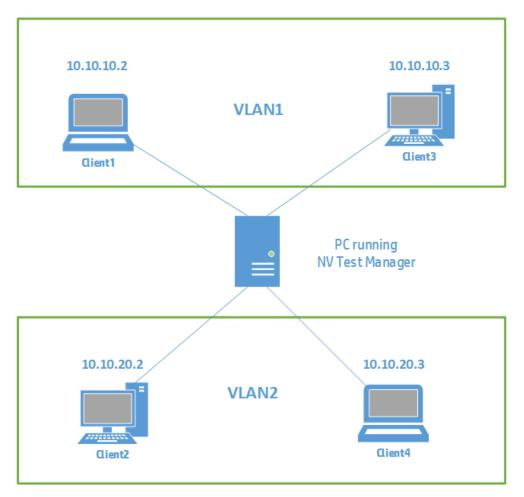
This configuration also enables routing between VLANs residing on the same physical segment (InterVLAN routing). NV impairs routed network traffic which uses the same physical port for both ingress and egress.
