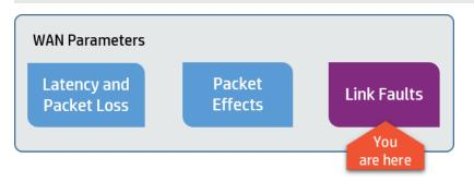
Link faults consist of effects caused by physical link malfunctions, specifically bit errors and disconnections. Bit errors are emulated by instructing the NV Test Manager to toggle bits at a given frequency. To achieve "disconnection" in the WAN Cloud, you can instruct NV Test Manager to stop responding for a given period. Click the **Link Faults** tab to set the parameters that help emulate the link faults.
