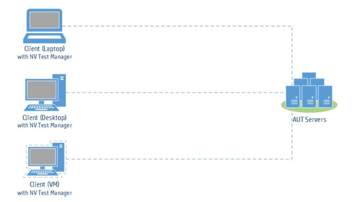
Configuration 1 can also be used in conjunction with Configuration 3. In the following diagram, the testing environment is running on a hypervisor. NV Test Manager is installed on each client VM in order to add the required network conditions between the client and the AUT servers. In addition, NV Test Manager is installed on a VM configured as a router between the AUT server and the DB server, for adding the network conditions between them.
