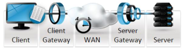
When you create an Advanced Test, you add flows to the test. A flow is a set of network impairments and conditions that are applied to network traffic that flows between the **client**<sup>1</sup> and **server**<sup>2</sup> IP addresses that are defined in the flow. You may need multiple flows in a test if a client communicates with multiple servers, and there are different latencies for each server.
