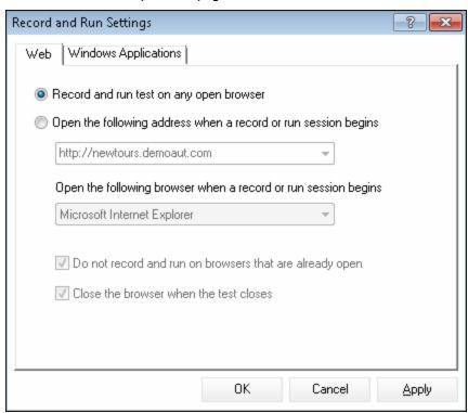
In the **Web** tab, select **Record and run test on any open browser** and click **OK**. This enables UFT to record on the open Web page.
