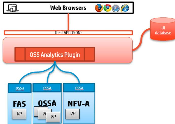
Figure 3 – Multiple servers configuration for OSSA Plugin
