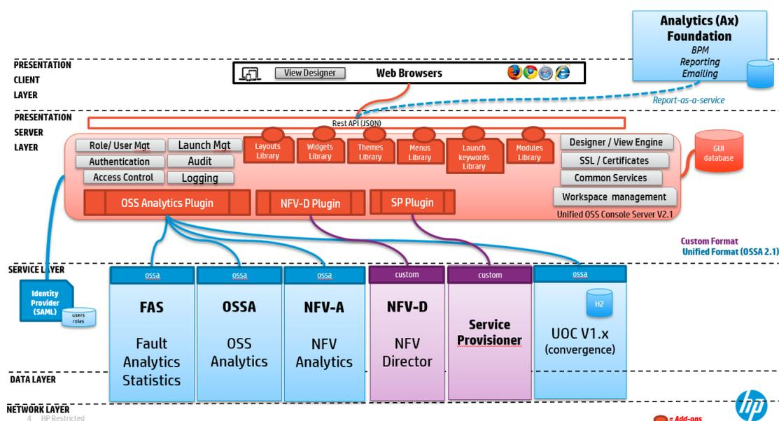
Figure 1 – UOC V2.1 High level architecture
