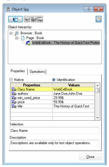
When you are ready to create a test on the control, the **Select**, **GoToAuthorPage**, and **GoToUsedBookPage** methods are supported. These methods can be recorded or you can select them manually in the **Operation** column of the Keyword View. When recording a test, both clicking on the book's image and clicking its title result in a **Select** step being recorded.
